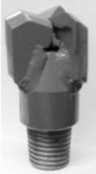
Chevron bits are designed for medium to hard formation and are used in areas that contain a lot of rock and also in the oilfield for drilling out concrete casings and plugs.
