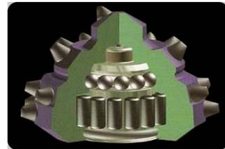
2.) STANDARD OPEN BEARING ROLLER BIT FOR AIR DRILLING: Cones are similar to #1, but have air injection directly to the cones to cool the bearings. Air flows into the cone through the passage ways inside the pin. (Not for mud applications)
